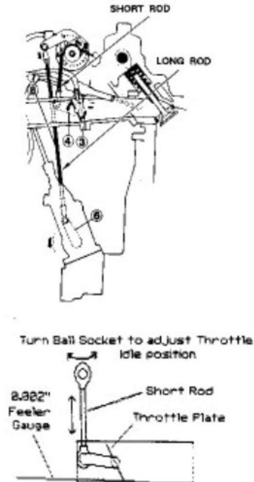
B.) Use a screwdriver to slightly turn the synchronizer screw between the two throttle shafts. Check the throttle openings with feeler gauges after each adjustment. The tension on both feeler gauges can change as the synchronizer screw is turned, so make sure that you check both throttles after each turning of the screw. When the throttle plates are correctly synchronized, the same tension is needed to pull a feeler gauge from any of the throttles.
